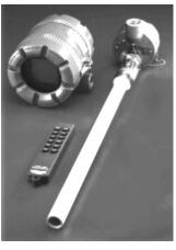
Model 4081FG's oxygen probe and electronics ARE **INTRINSICALLY SAFE** without requiring costly design modifications such as flame arrestors. The oxygen probe is constructed of ceramic materials capable of withstanding the higher process temperatures. Also, the analyzer eliminates the use of the cell heater, using the higher process temperatures to heat the zirconium oxide sensor cell to the temperature required by the
